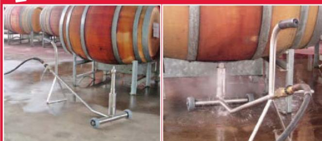
The New URC-HD model provides the same cleaning efficiency as its predecessor the well known Type URC, however, without the need for electric power supply and flexible drive shaft system.
